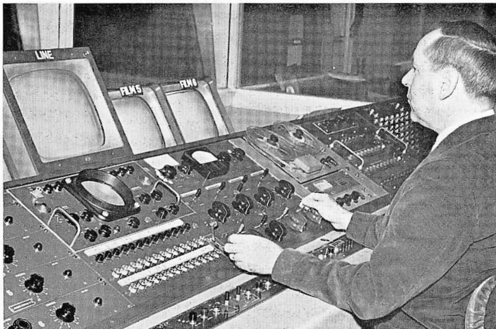
FIG. 5. Grant H. French at the control position of KOOK-TV's 12-input TS-40 Switcher.
