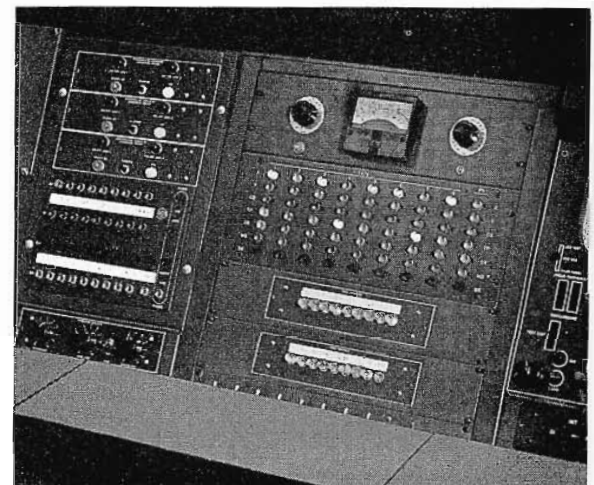
FIG. 10. Central control position of main console. Here all equipments can be put into the record mode, monitored and switched.
