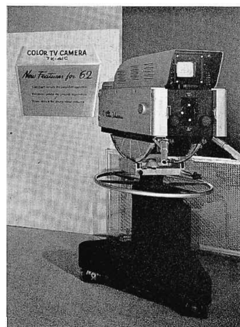
FIG. 3. TK-41C color TV camera, standard of the industry. New features for 1962 include stabilized circuits for simplified operation, precision yokes for precise registration, and prism optics for sharp clear color pictures.
