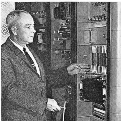
FIG. 1. *L. L. Caudle, Jr., inspecting cross point groups of TS-40 Switching System.
