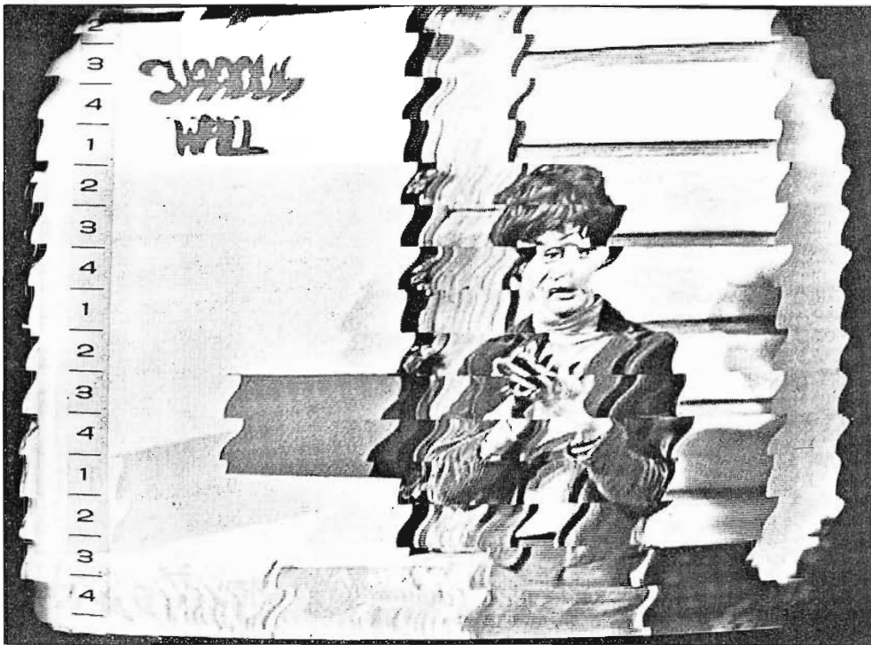
FIG. 23. Photograph of a tape playback taken from the recorder monitor with tip penetration mis-set. The picture exhibits excessive skewing.
