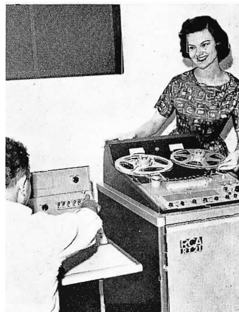
FIG. 9. RT-21 Stereo Tape Recorder in new console mounting gives top quality stereo performance. Also includes special stereo features such as module amplifiers and provision for extra stereo playback head.
