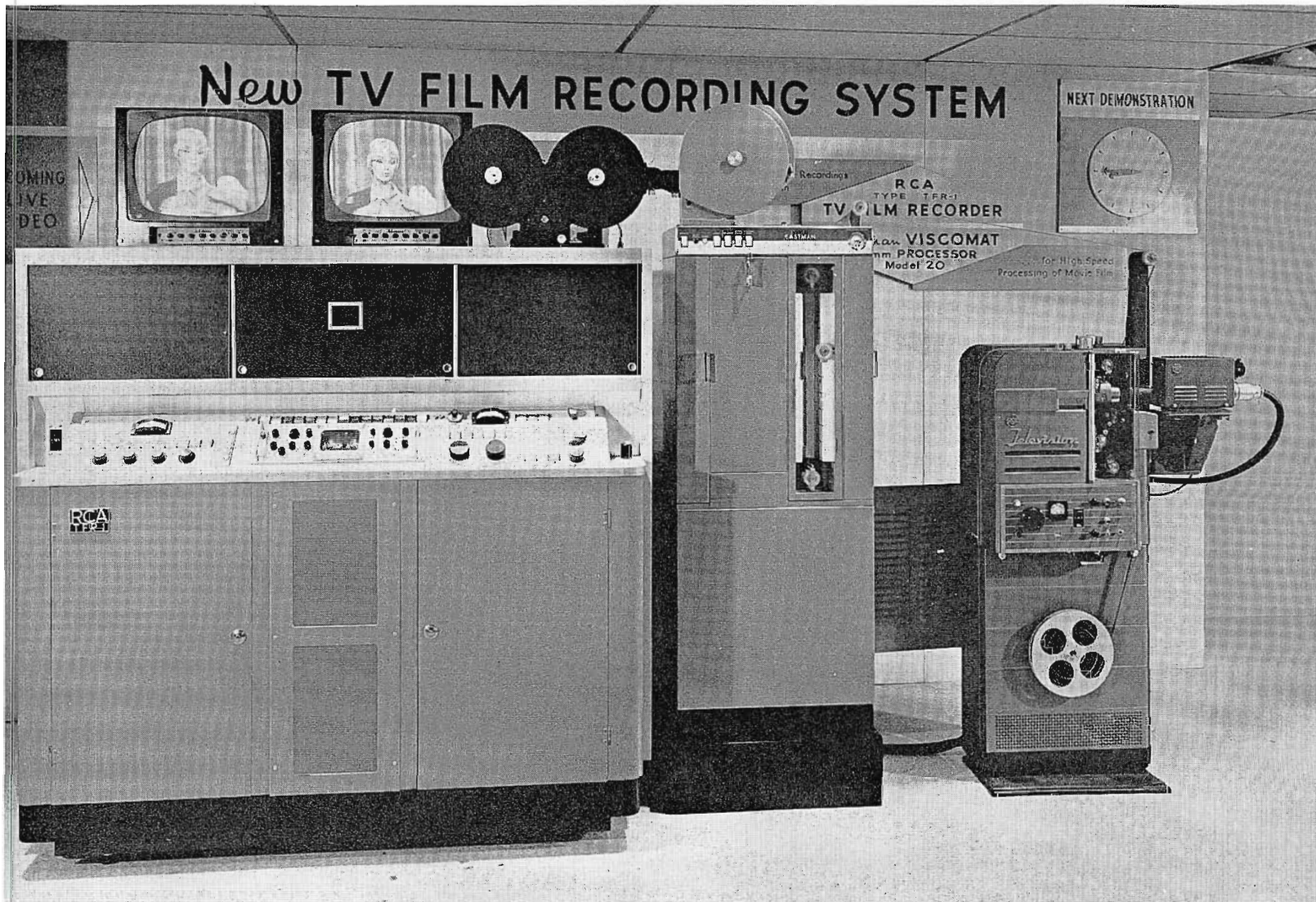
FIG. 7. Television film recording demonstration. TV pictures were recorded on film and played back through a TV film system in less than two minutes. Left to right are TFR-1 film recorder, Eastman Viscomat hot processor, and TP-6 projector with TK-21 Vidicon film camera.
