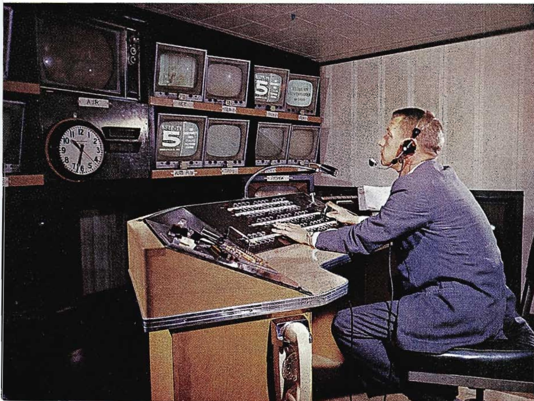
FIG. 9. One of two master production control rooms. These are equipped with TS-40 Transistorized Switching and RCA Special Effects Systems. They can handle both color and monochrome programs.
