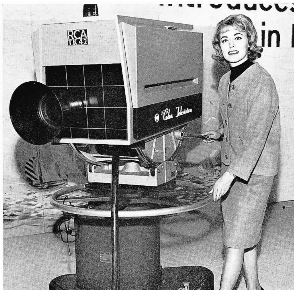
FIG. 2. TK-42X experimental M-Channel color camera. The new camera uses four tubes to produce richer hues in color pictures and for sharper black and white pictures. A single zoom lens replaces the familiar multi-lens turret.
