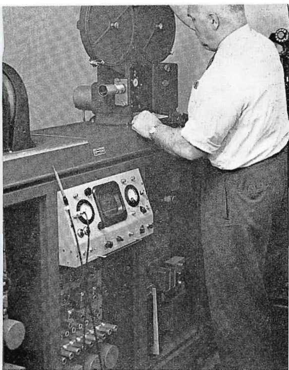
FIG. 11. Reeves kinescope recorder. Ken Jordan, kine operator. A second unit is being installed.
