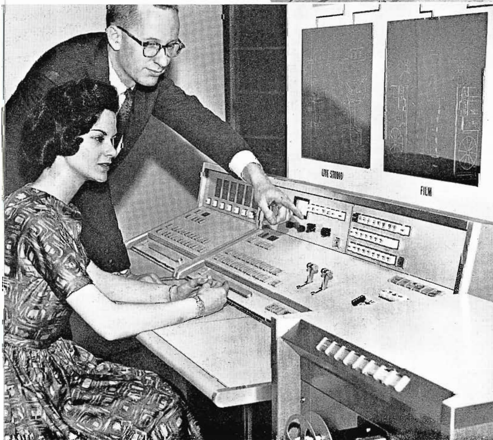
FIG. 5. TV's new control console handles all the station's switching operations, controls associated mechanical equipment, and can be completely automated by adding clock and memory units.
