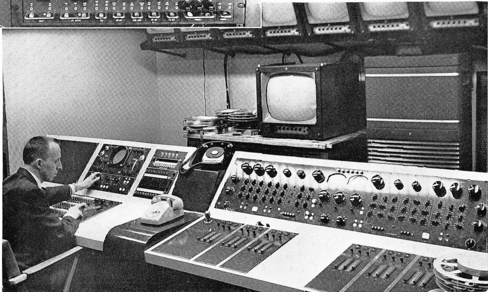
FIG. 22. Audio console (right) and video (left) of mixing studio Y, which is equipped identically to Studio X. Charles Power, maintenance engineer, is shown at TS-40 Transistorized Switcher panel.
