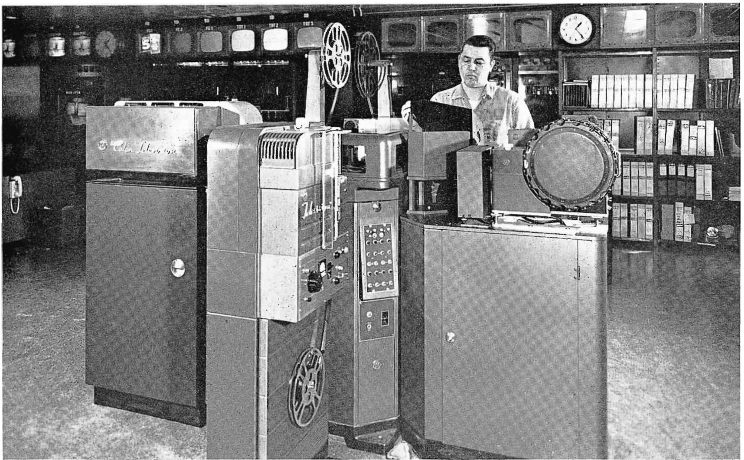
FIG. 40. Don Kline, projectionist, at Film Island No. 1 which includes two TP-6 16mm projectors and a TP-7 slide projector. Also TK-26 Color Film Camera, TP-15 Multiplexer, and TK-21 B & W Film Camera.
