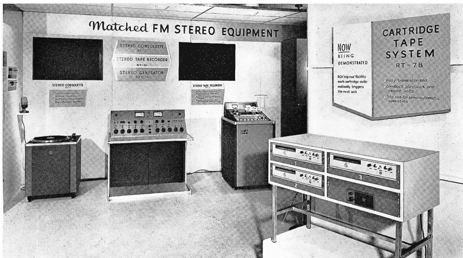
FIG. 8. Matched FM stereo equipment including (left to right) BQ-2C Turntable with Universal Pickup Cartridge, BC-7 Stereo Console and RT-21 Stereo Tape Recorder. In foreground is RCA's transistorized cartridge tape system.
