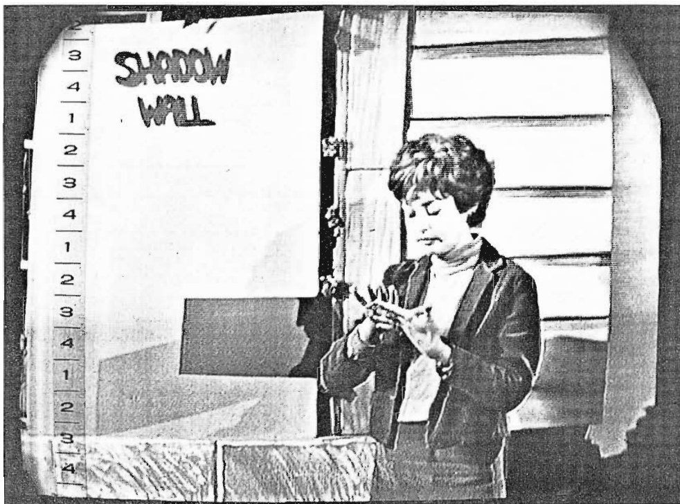
FIG. 23A. The same monitor photograph as in Figure 23 after processing by the ATC unit. All geometric errors have been removed.
