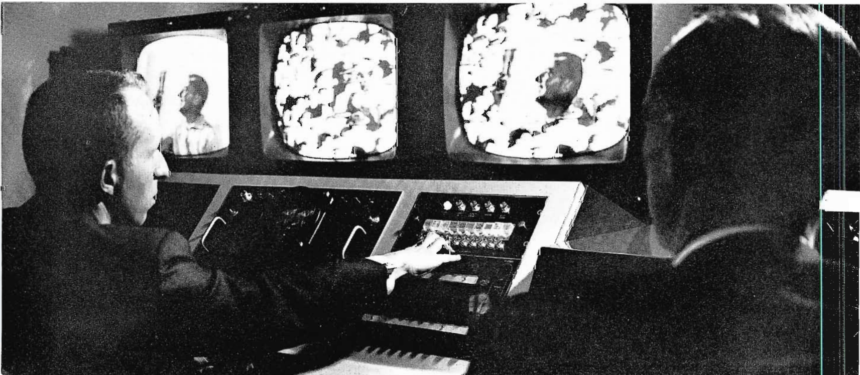
FIG. 28. The RCA special effects control panel in operation at Studio X. Note effects produced as shown on monitors.
