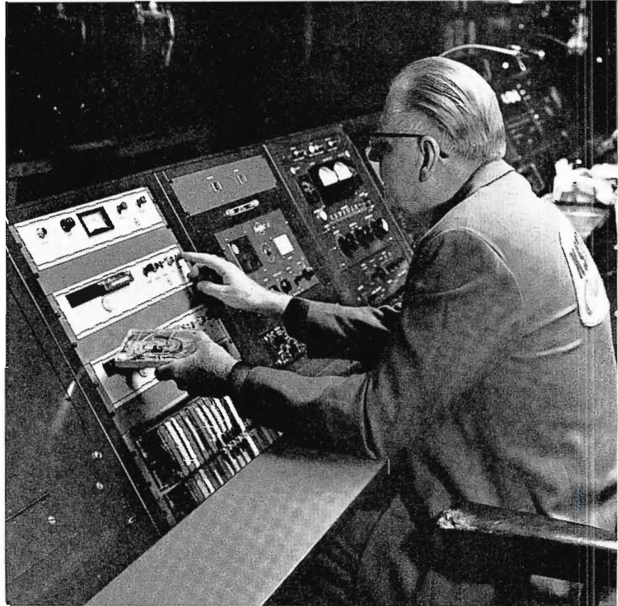
FIG. 26. RCA Cartridge Tape installations at master control. These units are tied into the automation system. Announcements are pre-recorded and started automatically for use with film and slide video. Ray Aula is loading a tape cartridge into the system.
